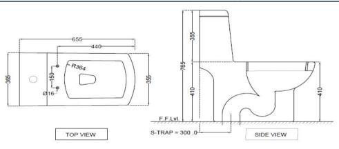
ALL DIMENSIONS ARE IN MM. (TOLERANCE ± 5 MM)
