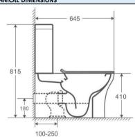
ALL DIMENSIONS ARE IN MM. (TOLERANCE ± 5 MM)
