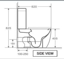
ALL DIMENSIONS ARE IN MM. (TOLERANCE ± 5 MM)
